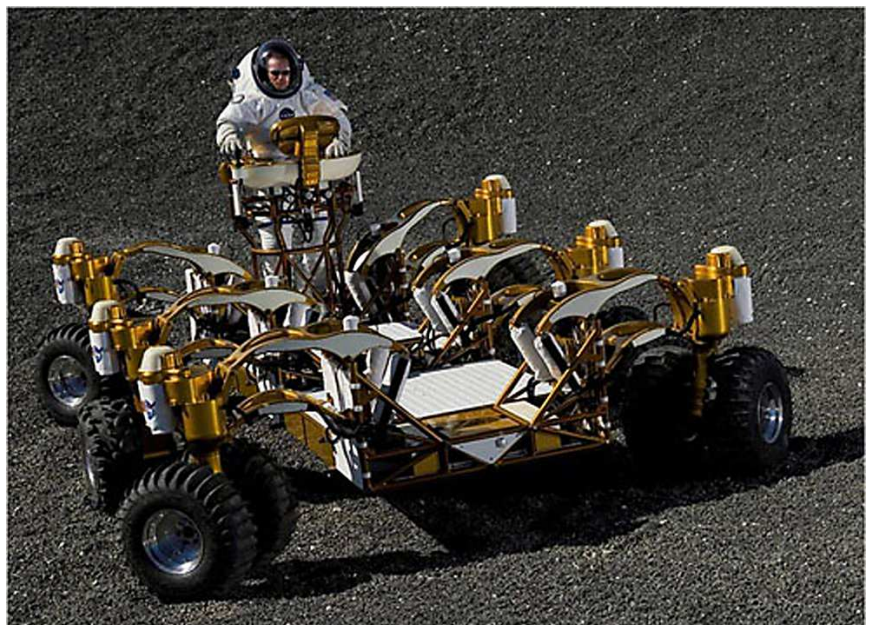
The Chariot Lunar Truck is one idea for a vehicle equal to the lunar terrain. Each of the six wheels pivots in any direction, and two turrets allow the astronauts to rotate 360°.
